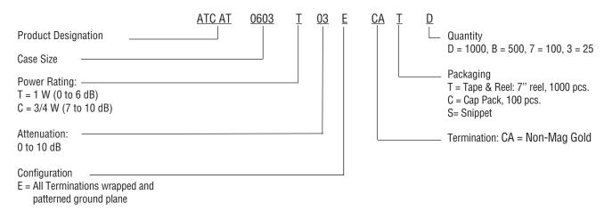
The above part number refers to an ATC AT 0603 Case Size with an attenuation of 3dB, 1W Power Rating, wrapped and patterned ground plane configuration with Non-Mag Gold Termination and tape and reel packaging, 1000 pcs.
